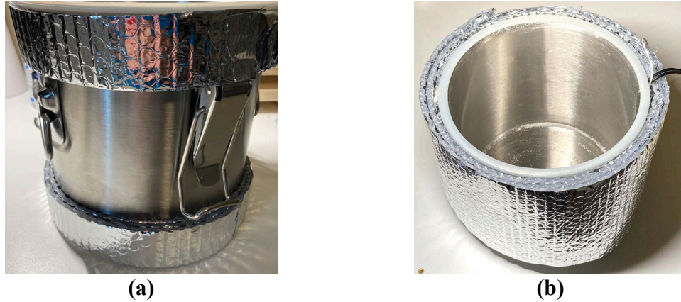
Figure 3.6. Install insulation on the chamber wall. (a) First, attach strips of insulation to build an air gap and span the protruding components on the chamber walls; (b) Next, install the large piece of insulation, fully covering the walls of the chamber.
