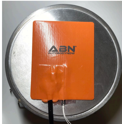
Figure 3.10. The heating element was adhered to the base of the chamber, with the thermistor secured on the interface.
