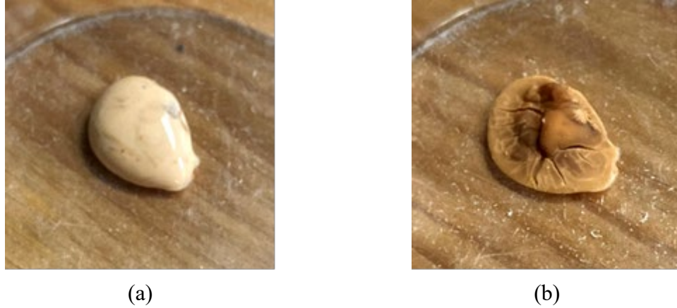
Figure 3.21. 500 mg samples of the consortium were dehydrated in a petri dish. (a) The wet culture, prior to drying; (b) The fully dehydrated culture.
