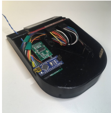
Figure 2.6. The LCD is held in place by two locators behind the slot for the screen. Its wires are tucked under a plastic wire manager attached to the TAL220 boss, then connected to the circuit board.
