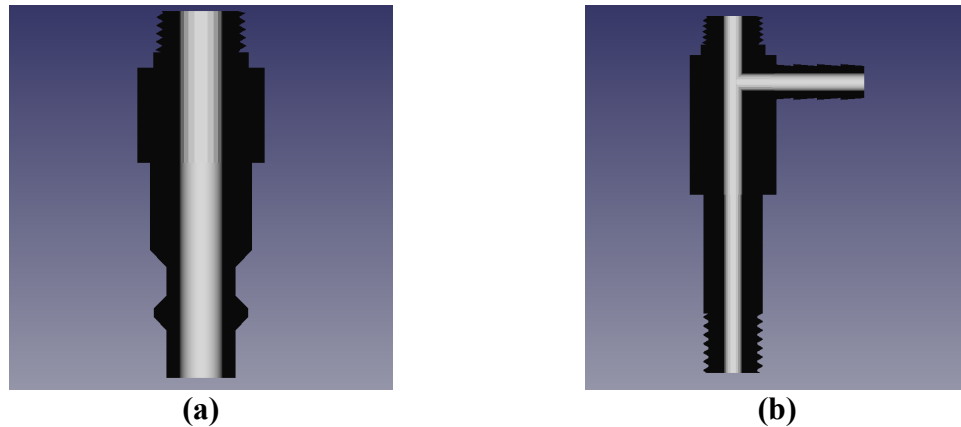
Figure 3.2. Air ejector connector cross-sections, highlighting internal geometry where air flows. (a) Intake connector, where high pressure air enters the ejector; (b) Vacuum connector, where evacuated air flows from the chamber to the ejector and vacuum pressure is measured.
